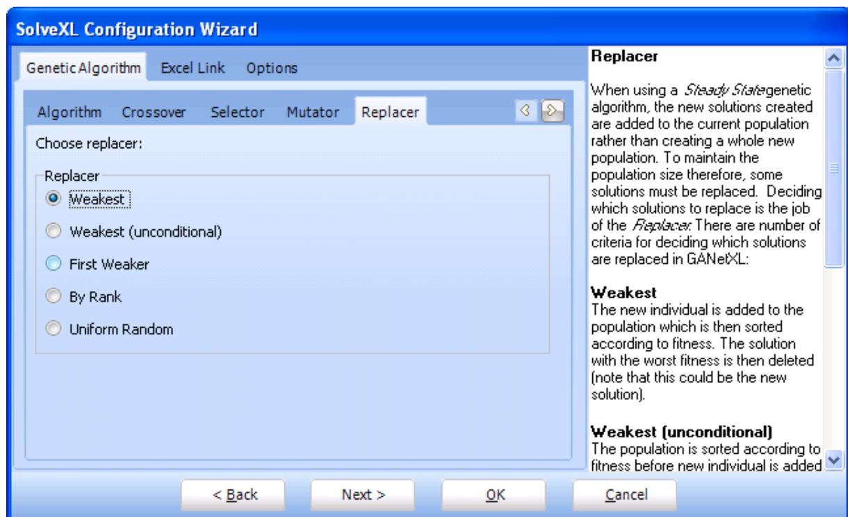
Figure 18 Choosing replacer used in SO Steady State
